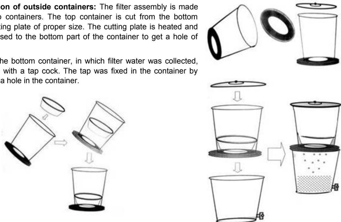
**Fixing of bed in the container :** Fixing the bed to the container is a very important step. The bed has to be properly fixed inside the container. The gasket of proper size was fixed over the bed and the bed with gasket was slowly and vertically inserted into the container. Once it was properly placed then the bed was pressed at
